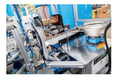
The DALEX system handles all tasks from cable feeding to measuring, cutting and stripping processes, feeding of the wire end contacts to welding of the contacts on both sides and ejection of the finished products.
