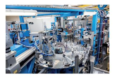
In order to produce the welding raw connectors in different cross-sections and lengths with repeatable accuracy in the shortest possible time and in high quantities, DALEX has designed a 16-station rotary assembly machine that is precisely tailored to the requirements.
