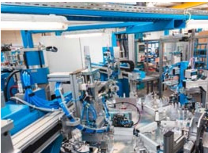
*Automatic rotary assembly machine for the fabrication of strand cables inclusive of reel units with dancer control, cutting the cable to length unit, designed & built for different cable lengths and diameters.*
