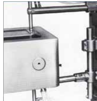
SWIVEL UNIT for welding hardt to reach spots:the electrode holder swive unit can turn on its axis and the lower arm can be adjusted in height.
