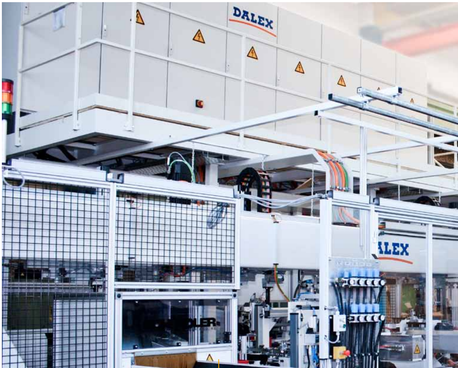
Linear transfer unit for fabrication of drawer side components
