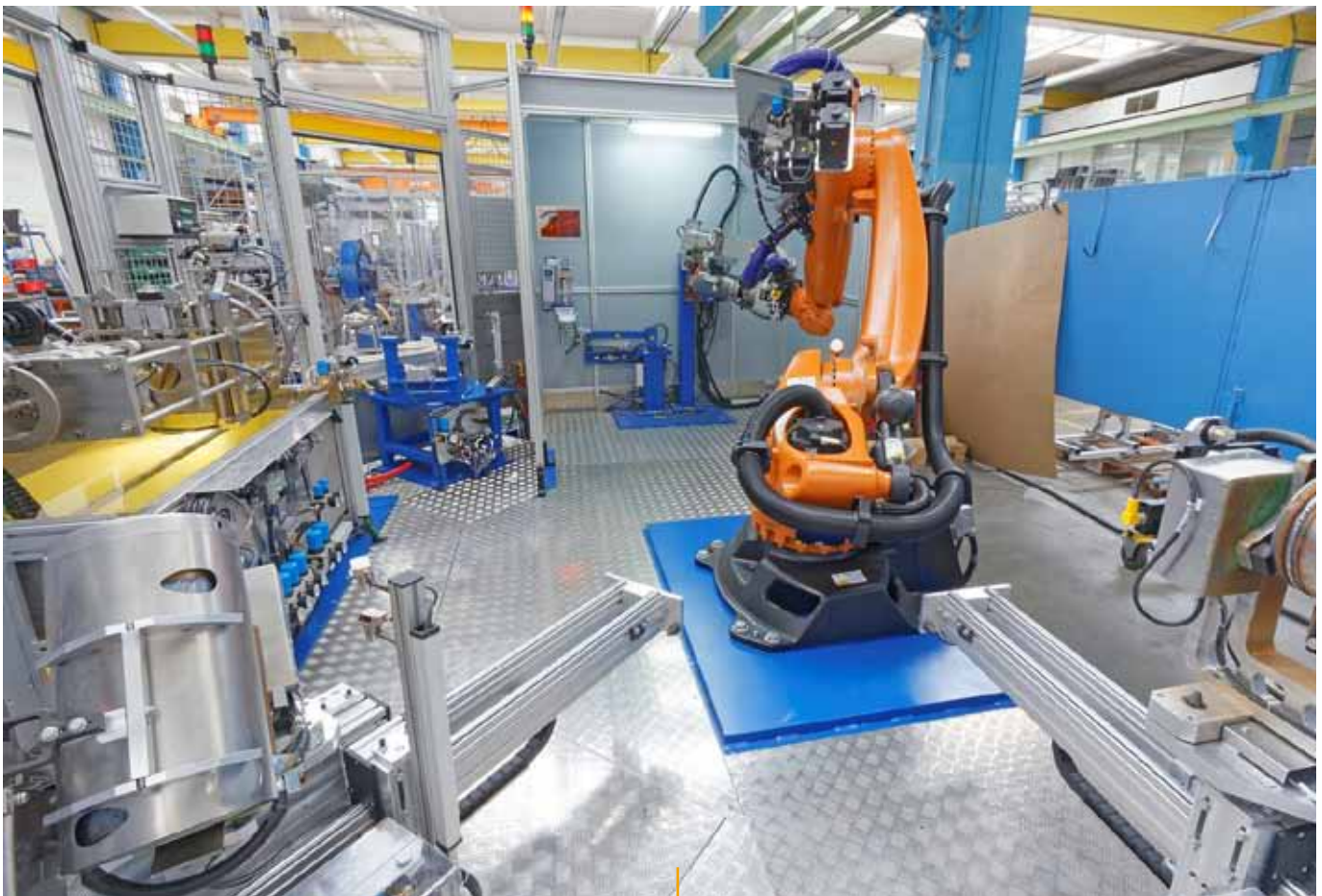
MAG welding of heat exchangers for truck auxiliary heating
