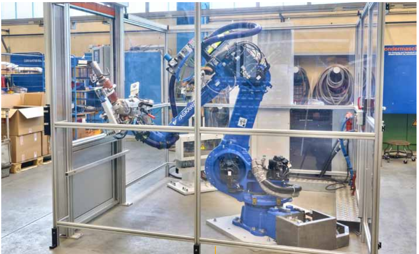
Handling robot with workpiece carrier
