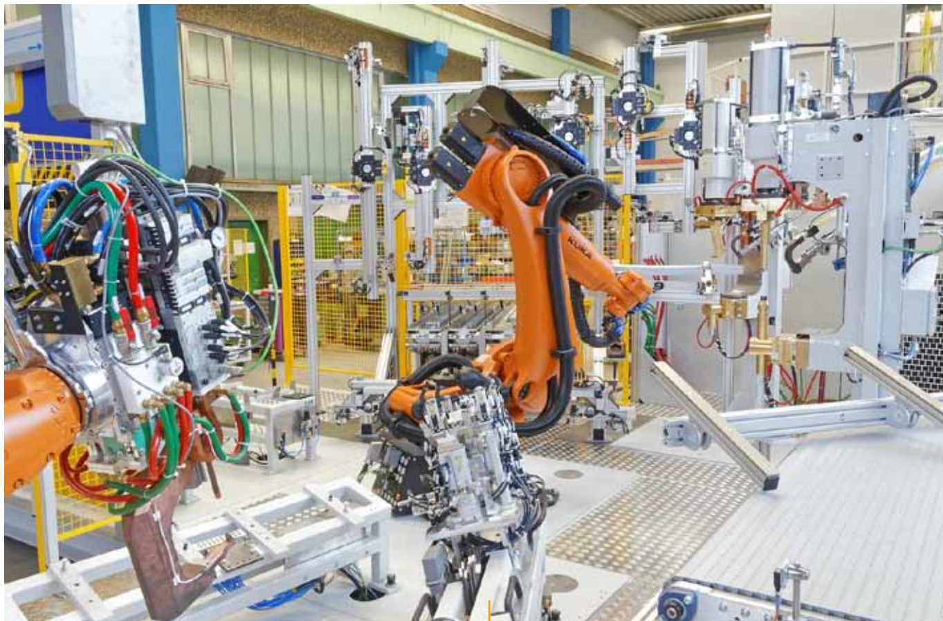
Robot welding plant with C modules..
