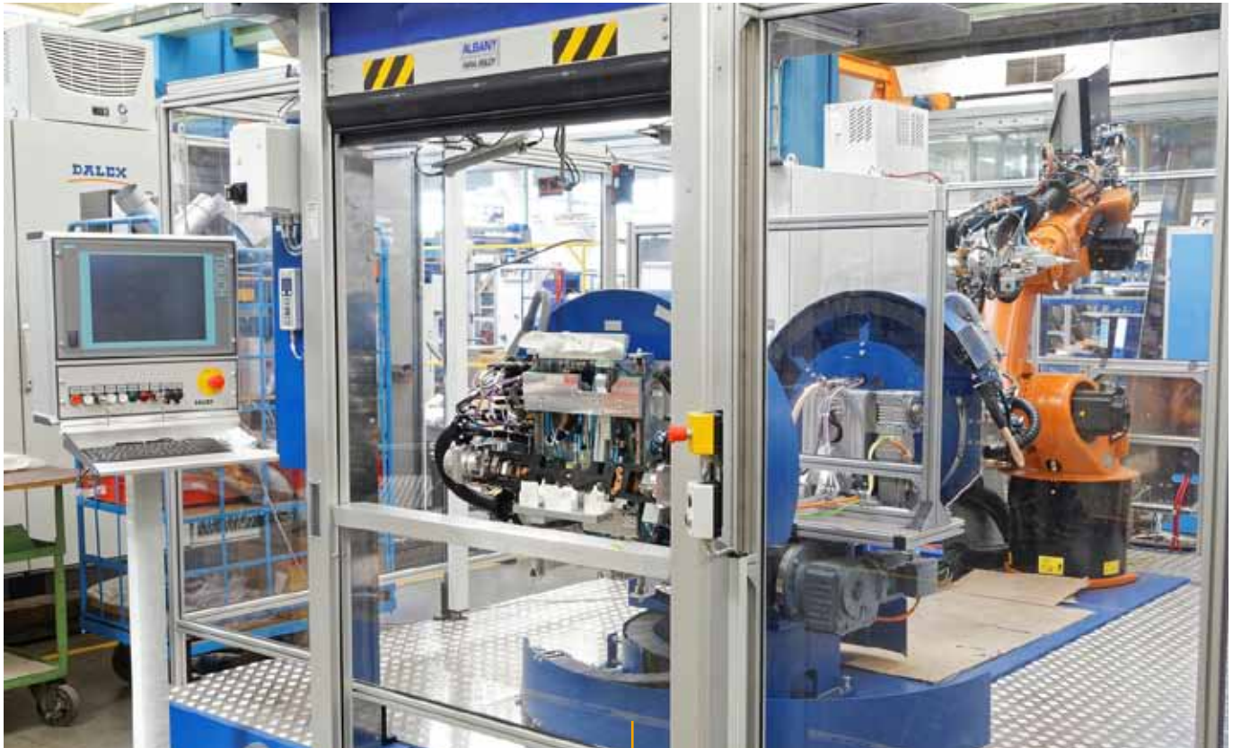
Robot in combination with rotary indexing table
