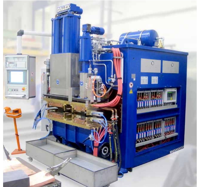
DALEX three-phase gleichstrom projection welding machine type PMS 38-6 G3 with 1200 (6 x 200) kVA
