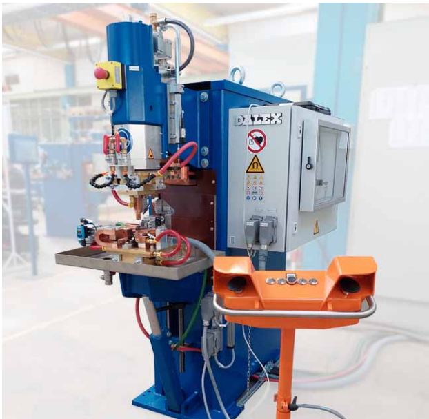
DALEX medium frequency projection welding machine type PMS 14-6 MF with 2 x 250 kVA
