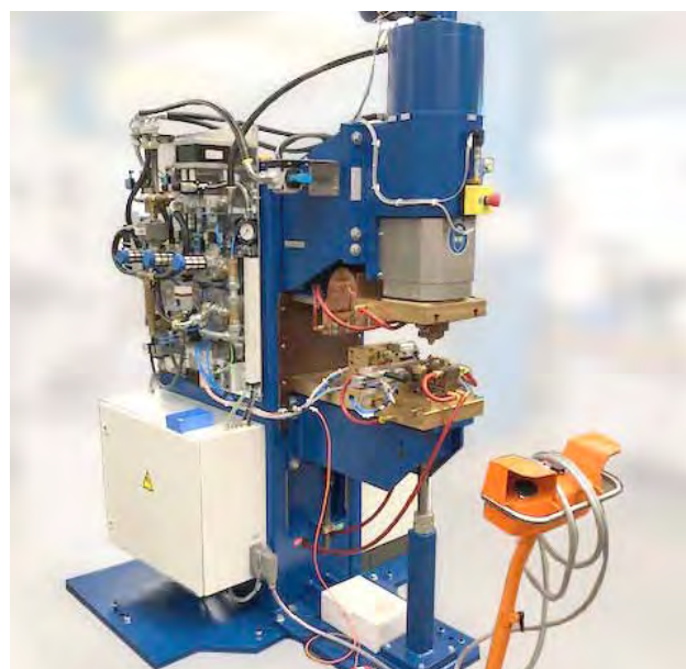
DALEX projection welding machine type PMS 36-6 MF in medium frequency technology with 700 kVA
