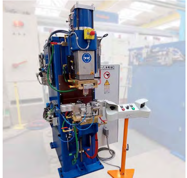
DALEX projection welding machine type PMS 36-6 MF in medium frequency technology 2 x 180 kVA
