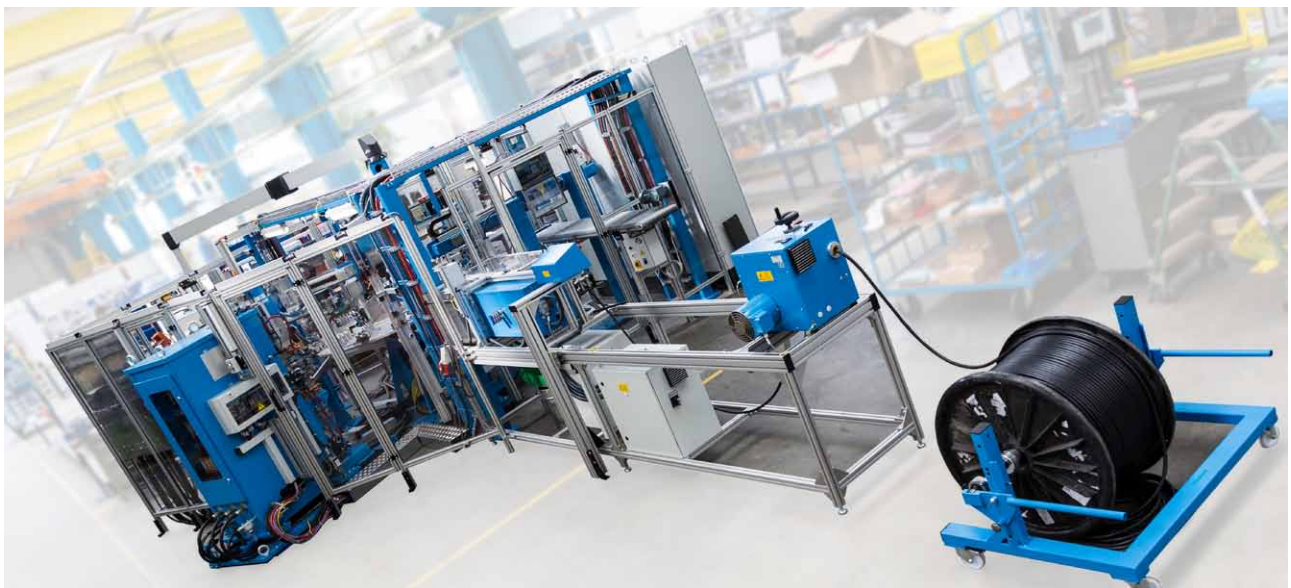
Fully automatic 16-station turntable system for cable assembly
