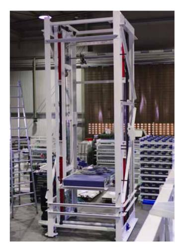
DALEX lifting systems transport pallets, pallet boxes, containers, etc. over several floors up to a conveying height of more than 20 m. Weights of up to over 2 t can be moved.
