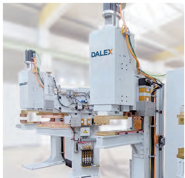
DALEX-C modules with projection welding armature in medium frequency technology, equipped with EPS drive 2700 daN
