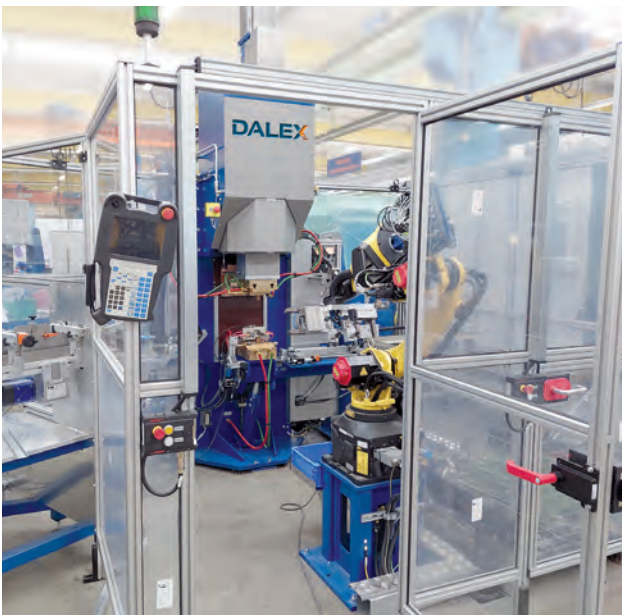
DALEX projection welding machine type PMS 37-6 MF in medium frequency technology, equipped with an EPS drive 4200 daN
