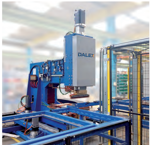
DALEX spot welding machine type PMS 12-6 MF in medium frequency technology, equipped with an EPS drive 2000 daN
