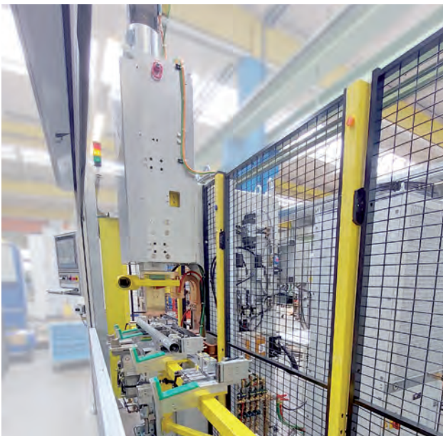
DALEX-C module as projection welding machine in medium frequency technology, equipped with an EPS drive 1750 daN
