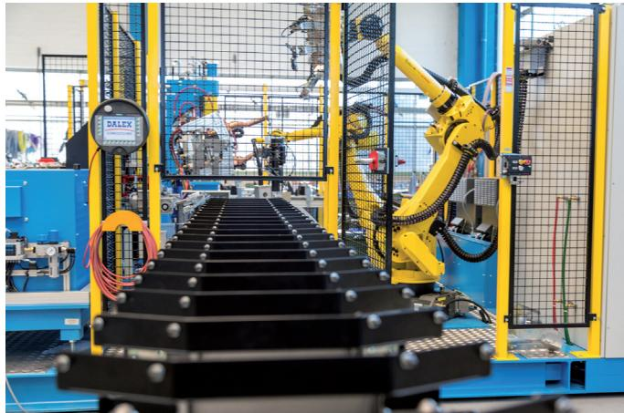
Semi-automatic and fully automatic feeding of the main product and small parts as well as downstream stacking and palletizing of the finished parts are an integral part of a complex overall solution.
