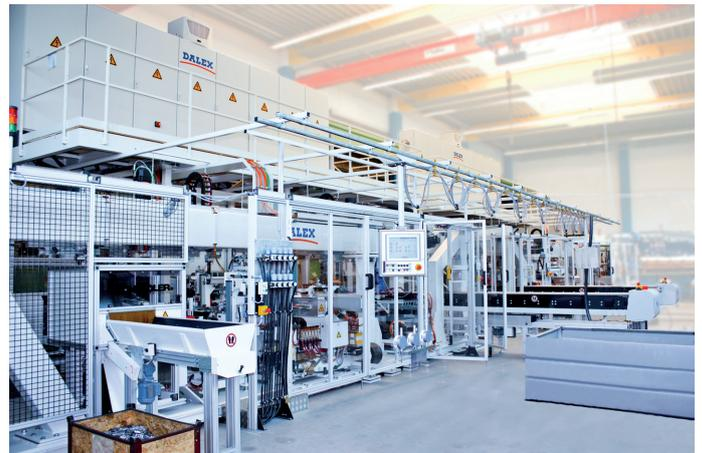
The fully automated overall solution from DALEX includes parts logistics, i.O/n.i.O. outfeed, mirror-image design for simultaneous production of left and right parts, and the space-saving control cabinet arrangement on a platform arranged above the system.
