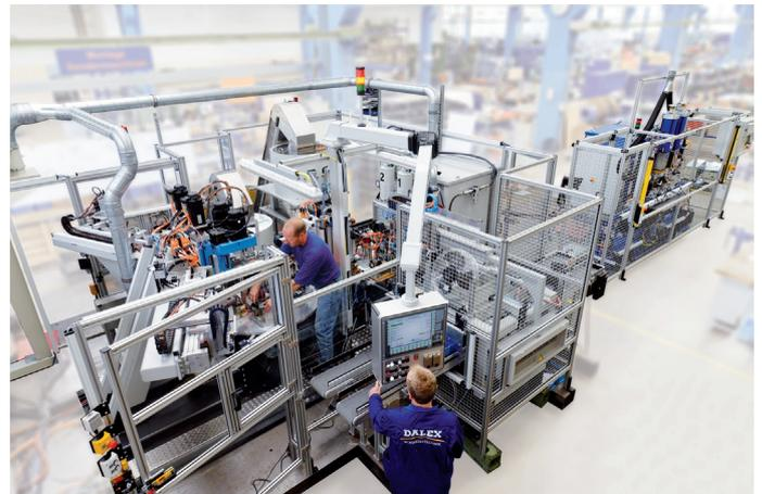
DALEX's highly complex production lines include not only welding processes, but also press-fit, testing and marking processes as well as upstream and downstream assembly steps.
