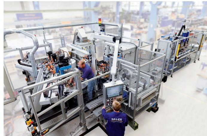
DALEX's highly complex production lines include not only welding processes, but also press-fit, testing and marking processes as well as upstream and downstream assembly steps.
