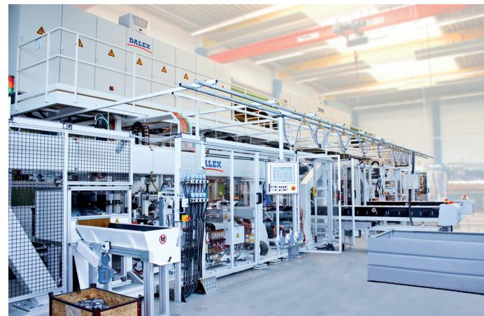
The fully automated overall solution from DALEX includes parts logistics, i.O/n.i.O. outfeed, mirror-image design for simultaneous production of left and right parts, and the space-saving control cabinet arrangement on a platform arranged above the system.
